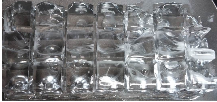
Figure 4.4 : A whole 3 by 7 ice block harvested from the cold plate during a preliminary experiment.
