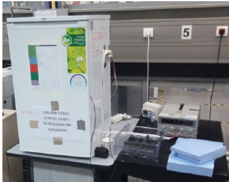
Figure 4.1 : The undercounter type refrigerator that was used as the cabin for the ice making device.
