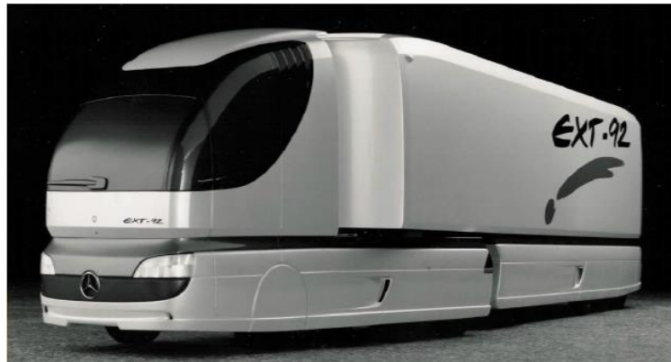
Figure 3.11: European Experimental Truck EXT-92, smooth side guard which redesign which diminishes the harm potential to vulnerable road users (Mercedes-Benz Australia)
