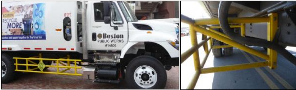
Figure 3.10: Frame mounted rail side guard
