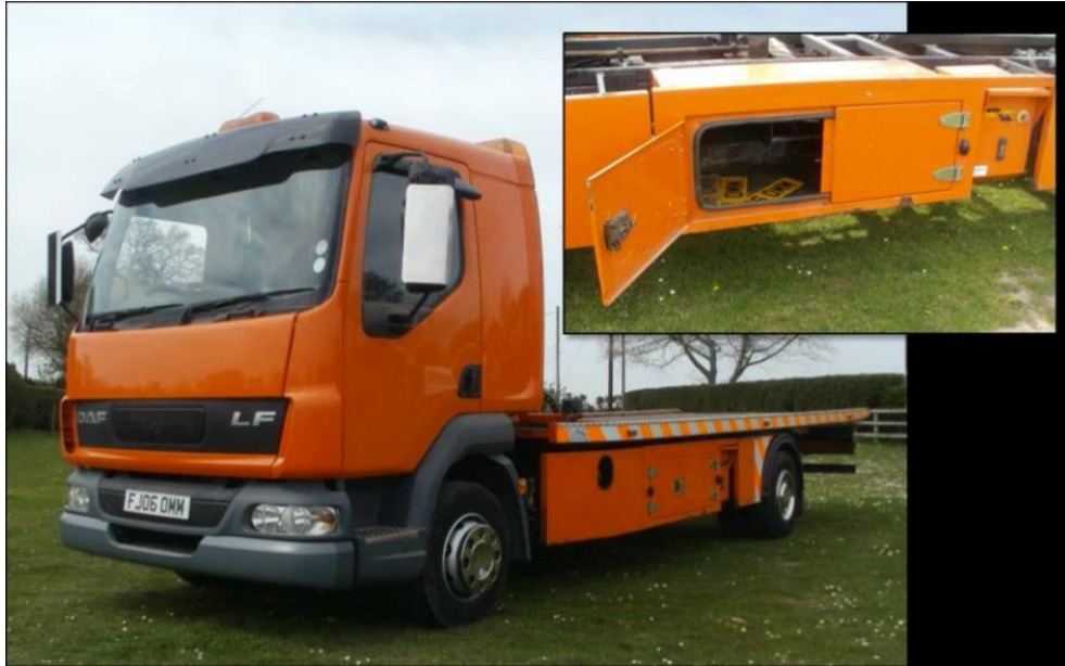
Figure 3.5: A side guard integrated in toolbox
