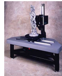
(c) Structured light scanner
