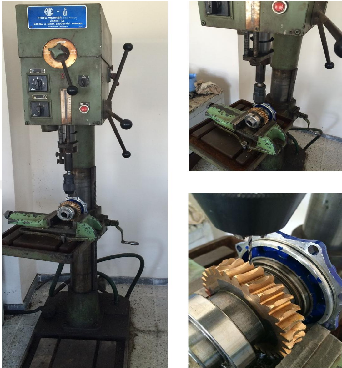
Figure 7.1 Simulated pits with a milling machine
