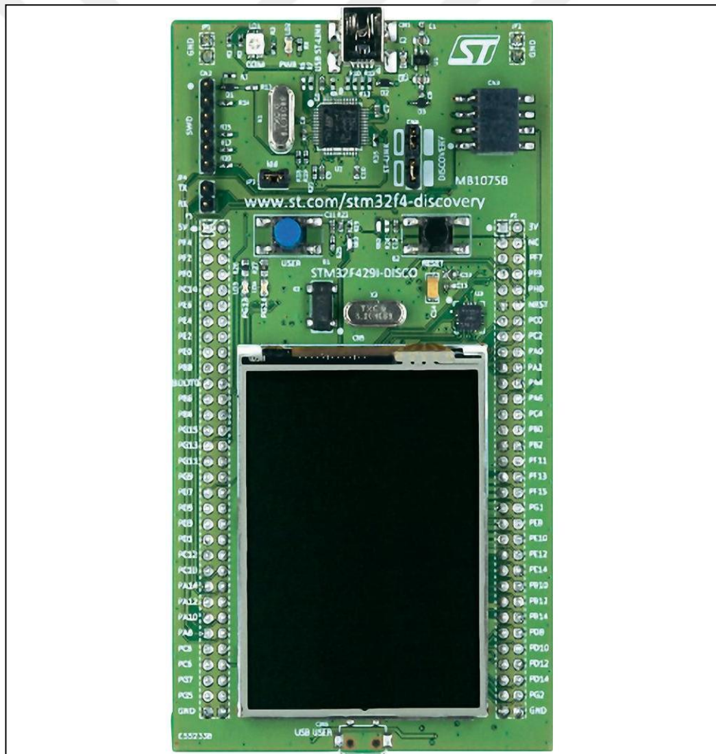
Figure 5.8 STM32F429 Discovery board (ST-STM32F429 Discovery Board, n.d.)
