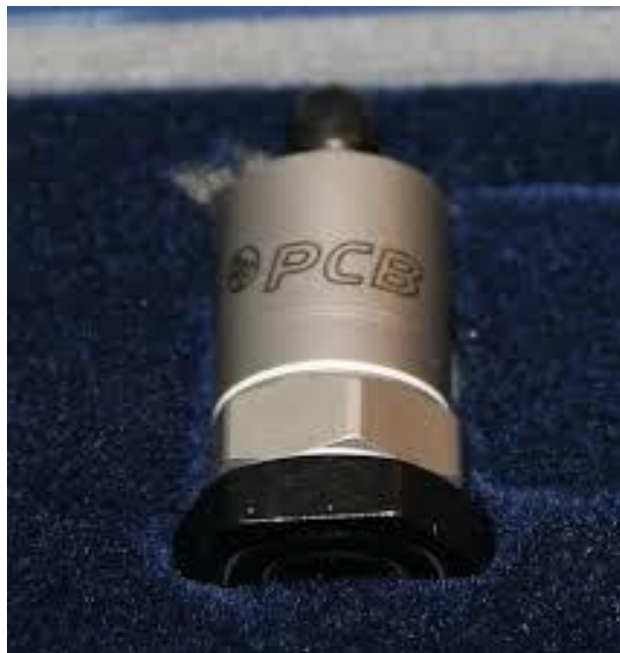
Figure 5.4 PCB Piezotronics brand 352A76 series accelerometer sensor
