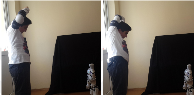
Figure 6.17. First stretching performance corrected by an appropriate feedback but wrong feedback was given to the second performance because of involuntary pose change of the body sensor
