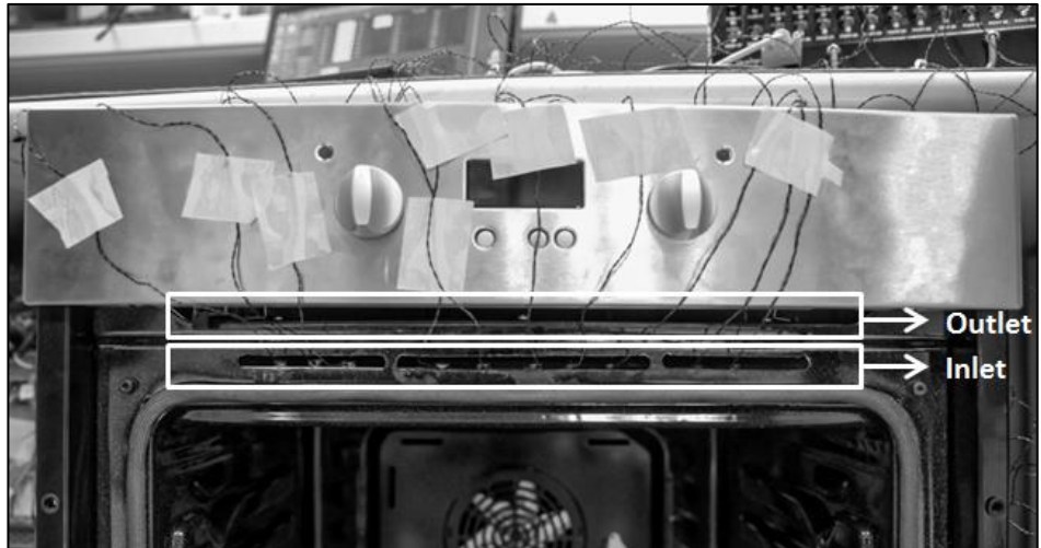
Figure 4.15 Arrangement of anemometers in experimental study
