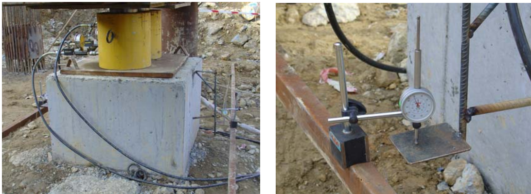
Figure 4.16. Reinforced concrete pile cap with reinforcement extensions for deformation observations
