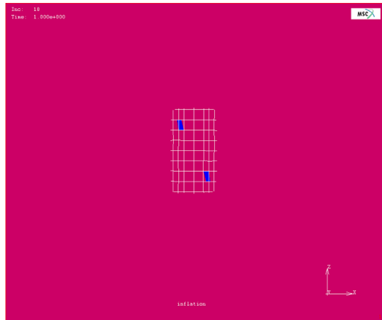
Figure 3.43. 25 mm (2393 N) deflected tire on a flat surface
