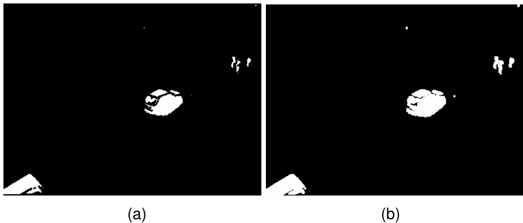
Figure 3.5 Effect of dilation operation, (a) Eroded image, (b) Dilated image (resulting image of morphological operations).
