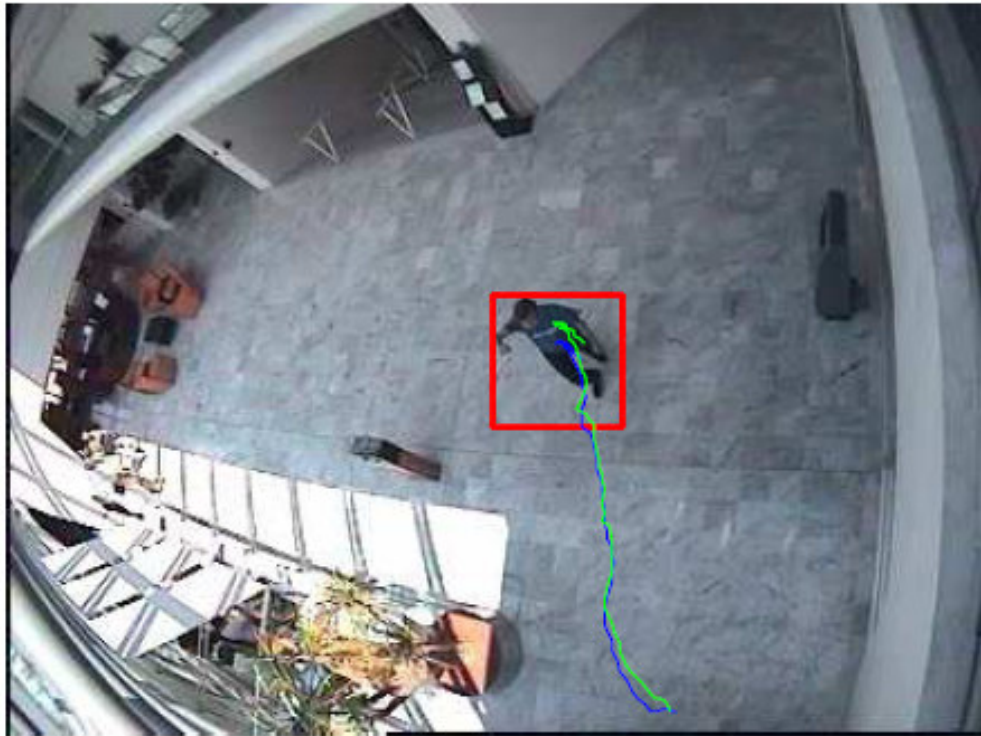
Figure 4.3 Kalman Tracker: Estimated and real trajectories of a moving object.
