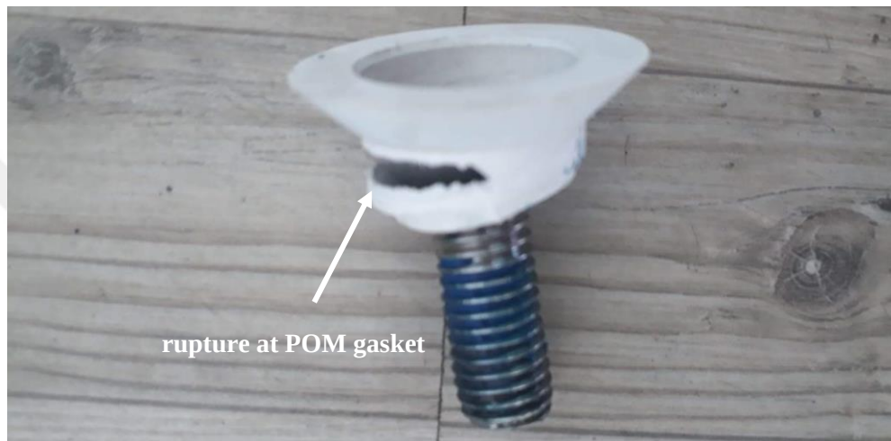
Figure 5.32 : Sample 3, plastic deformation of POM gasket of Glass Node.
