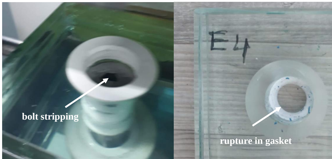
Figure 5.36 : Bolt stripping failure in Sample 4.
