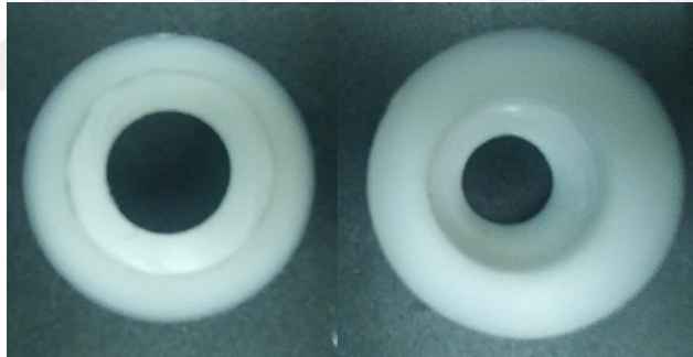
Figure 5.30 : First sample, deformed POM gasket of Glass Node.
