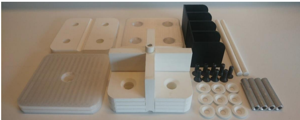
Figure 5.20 : 3D printed components of Glass Node
