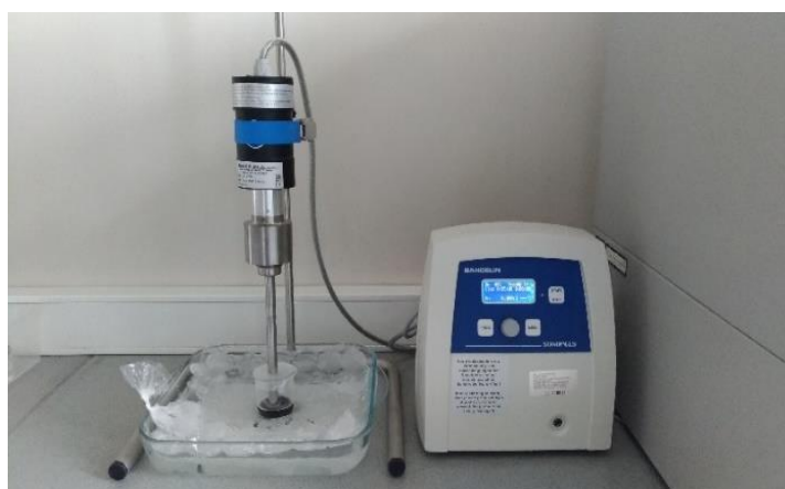
Figure 3.5: Sonication of CNT-SDBS-water mixture on ice-water bath.
