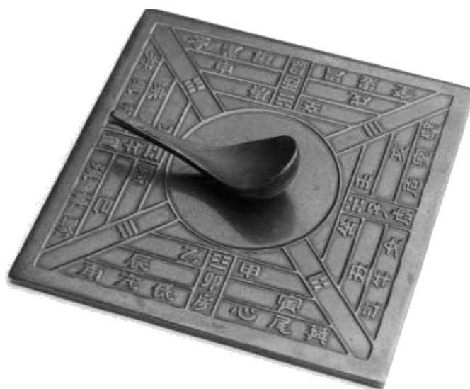
Figure 1.1: Magnetic compass spoon called Si Nan (Iron and Steel Research Institute, China, n.d.).
