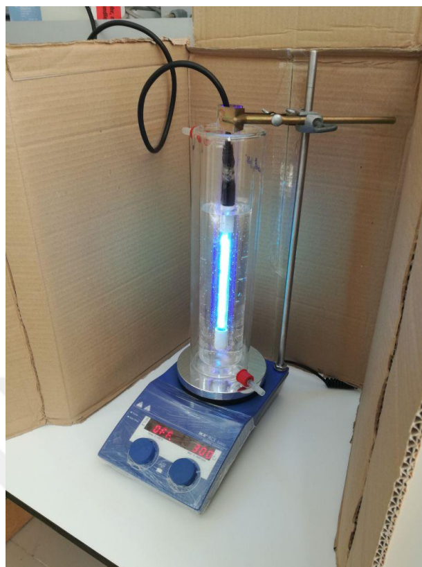
Figure 3.2. Experimental set-up used for Photo-Fenton and UV/ \text{H}_2\text{O}_2 Oxidation
