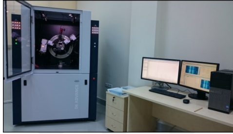
Figure 4.4. X-Ray diffraction (XRD) system (Bruker D8 Advance Twin-Twin)
