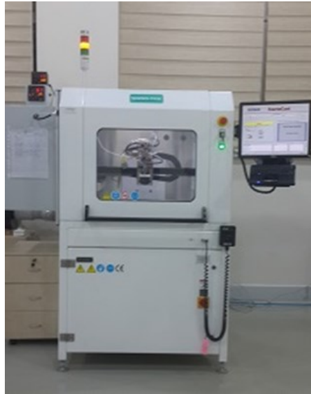
Figure 3.8. Ultrasonic Spray Pyrolysis system (USP)
