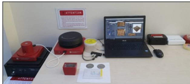
Figure 4.3. Atomic Force Microscope (Nanomagnetics ez-AFM)
