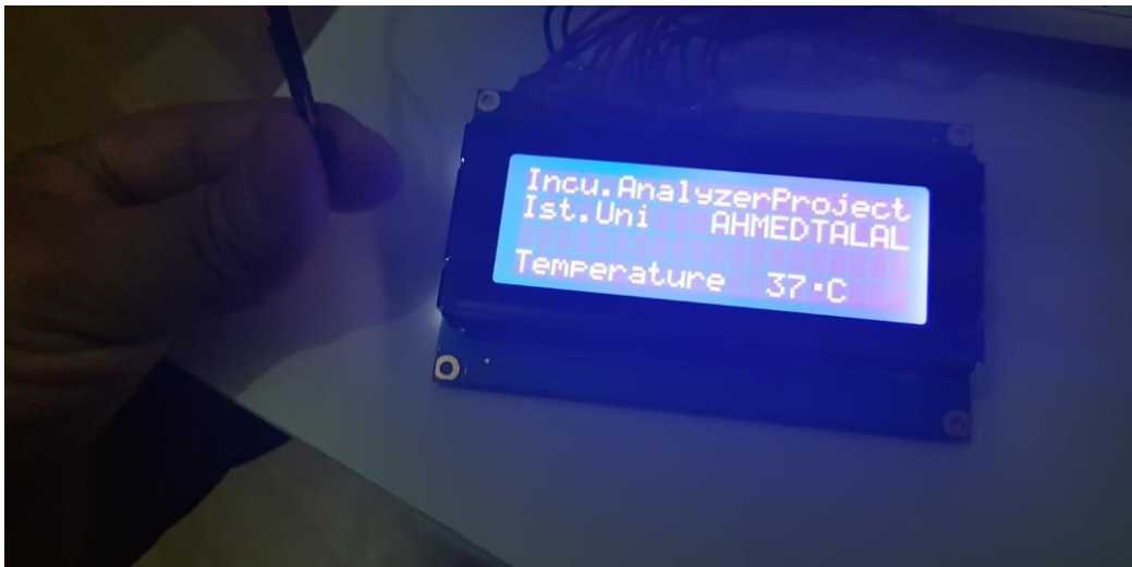
Figure 3.2: Measuring body temperature through LM35.
