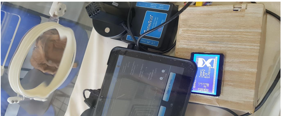
Figure 3.13: Testing our device in a Drager Isolette® Infant Incubator with a Datrend IncuTest incubator Tester.
