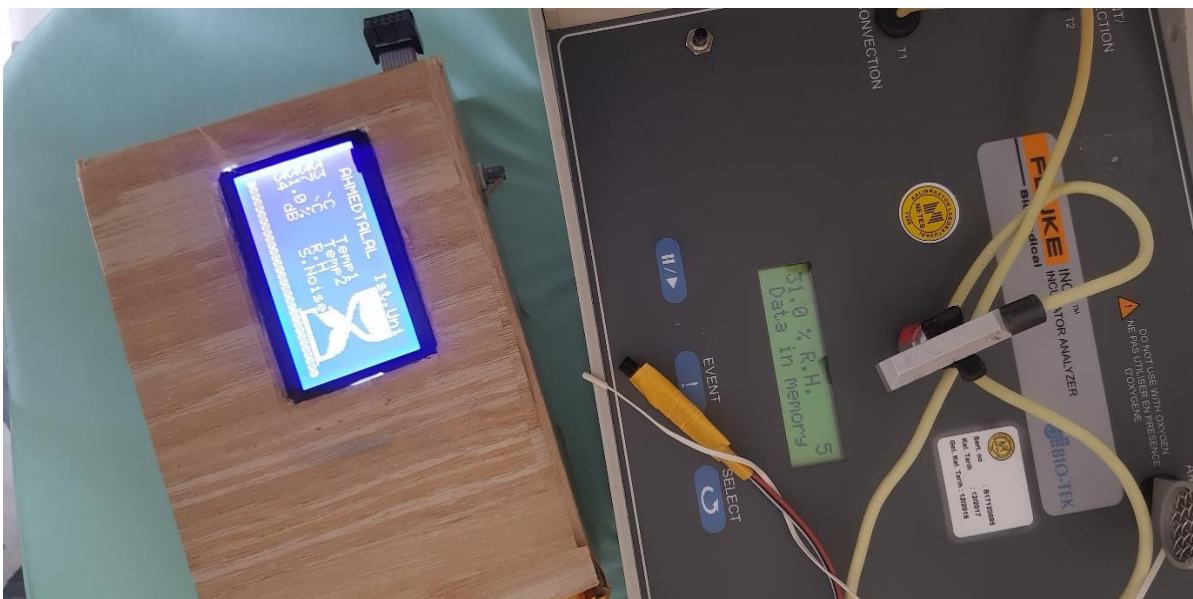
Figure 3.14: Testing our device in Girffe OmniBed Infant Incubator with a INCU Fluke incubator analyzer.
