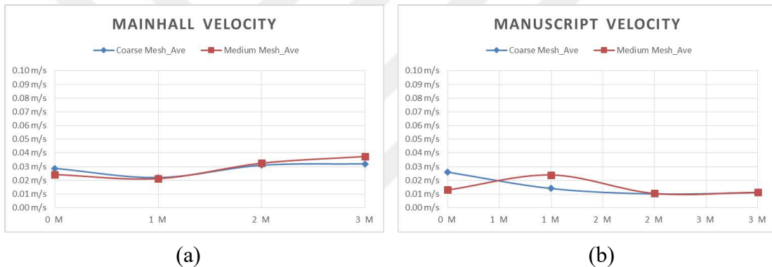
Figure 4.8. Average v change with height on (a) Main Hall and (b) Manuscript zones.
