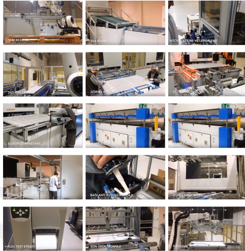
Figure 3.9: Panel Production Line [28]
