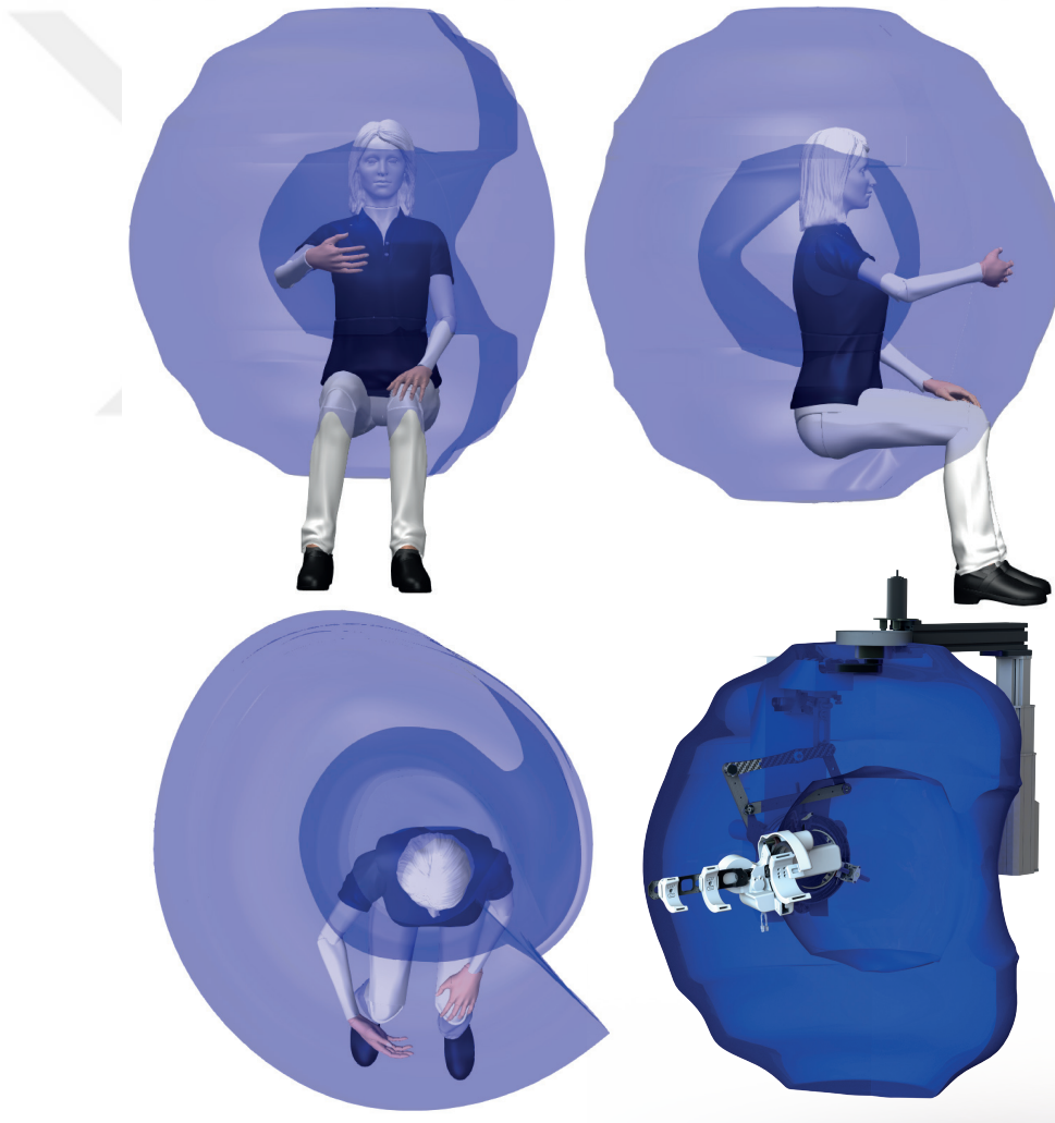
Figure 4.5: Top, side, and front view of the reachable workspace of ASSISTON-ARM at its end-effector
