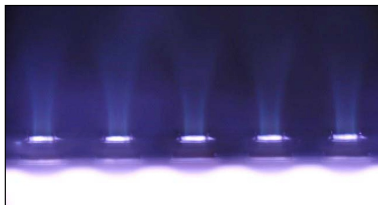
Figure 6.35: The experimentally observed well focused ion trajectories from a RF ICP ion thruster [13].
