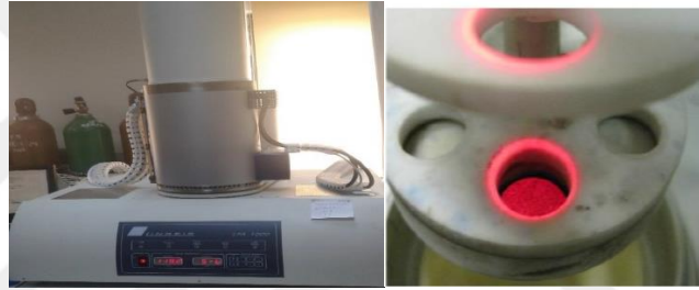
Figure 4. 10 : Equipment used for thermal diffusivity and specific heat determination.
