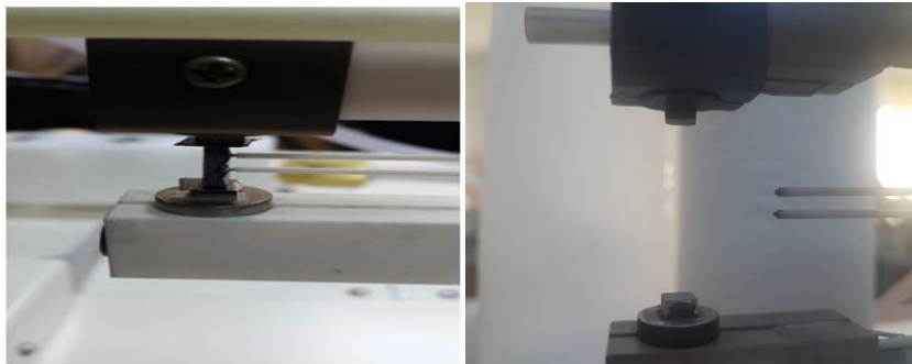
Figure 4. 9 : Measurement of resistivity and Seebeck coefficient.
