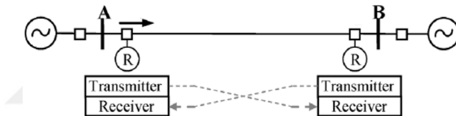
Figure 4.13 Communication scheme for directional comparison protection [30]
