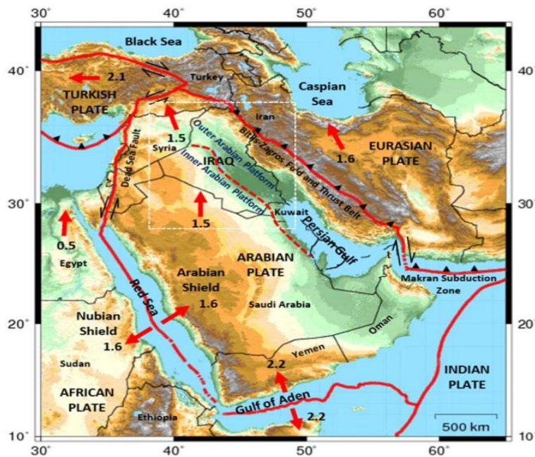
Figure 4.1 Tectonic setting of Iraq and environs (red arrows indicate plate motions in cm/year)
