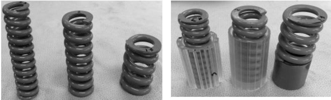
Figure 1: Test Springs with and without the inserts (LHL 1000D 05, LHL 1250D 03, LHL 1500D 01) www.leespring.com, Hefty Springs, Medium Load Series
