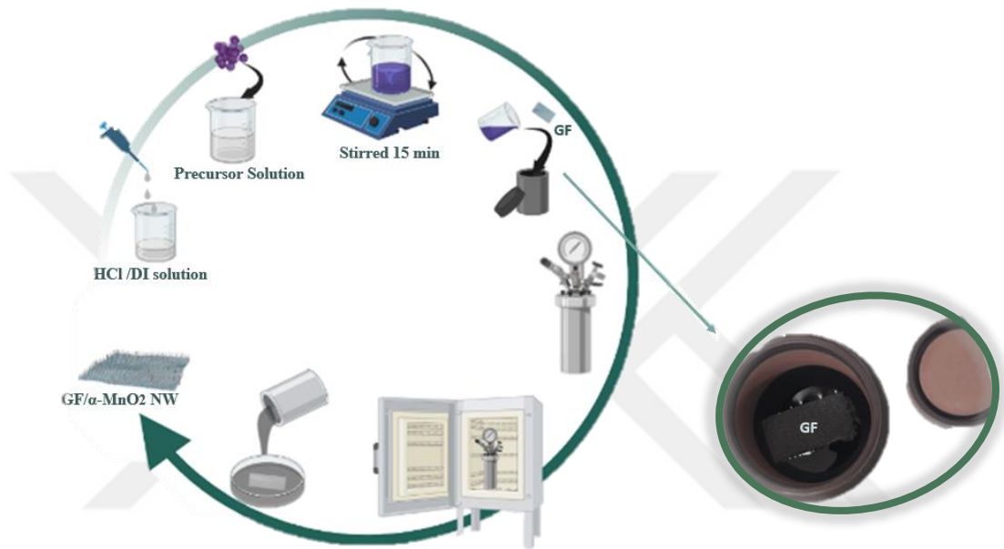
Figure 3.1. Graphical abstract of the MnO 2 NW growth via hydrothermal method
