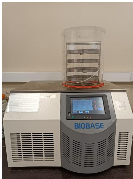
Figure 2.3: The lyophilizer device used for freeze-drying method
