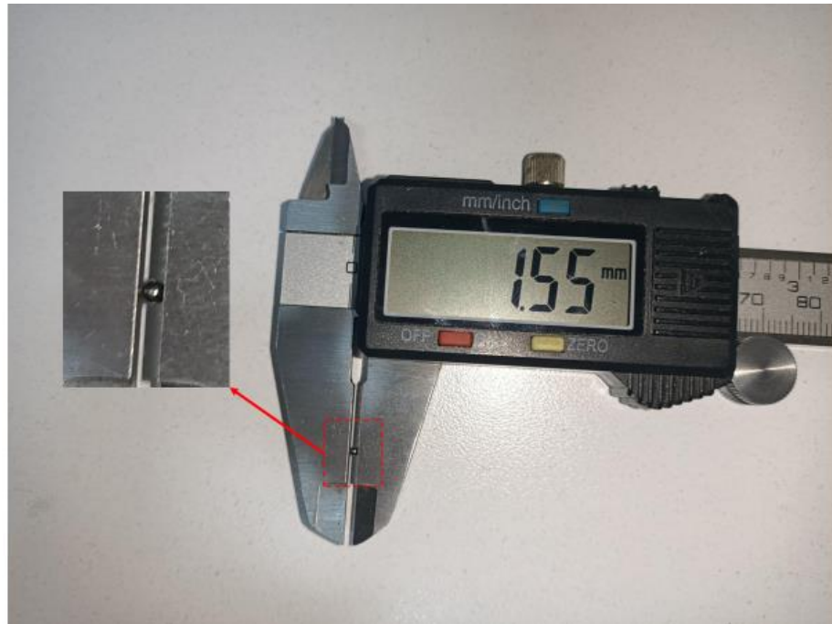
Figure 3.6: Micro robot and dimension
