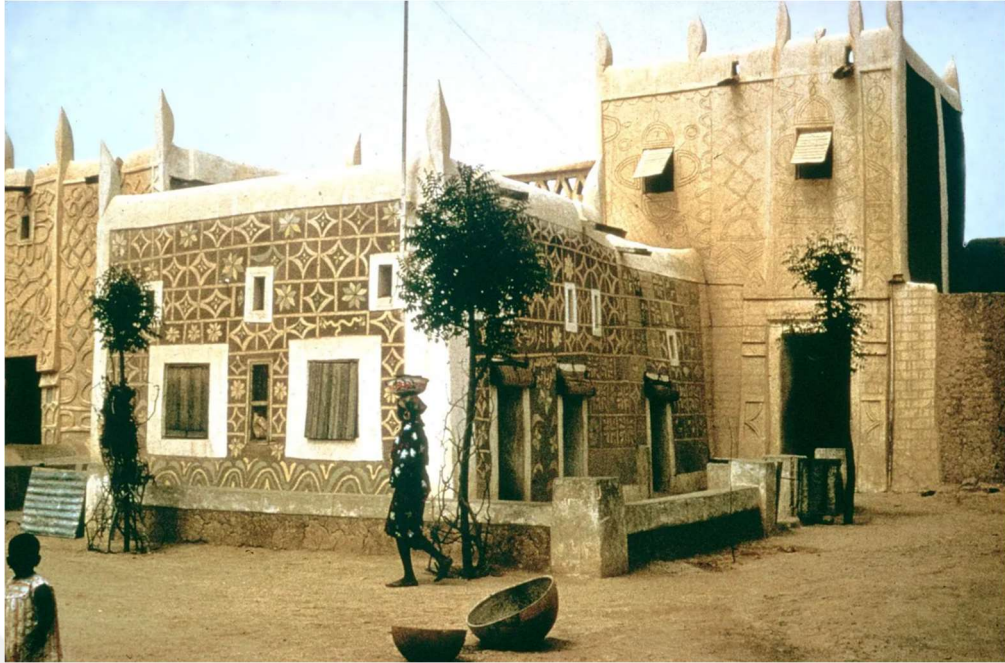
Figure 25. Zanko as seen on the roof of Gidan dan Hausa house in Kano (Samuel, 2022).
