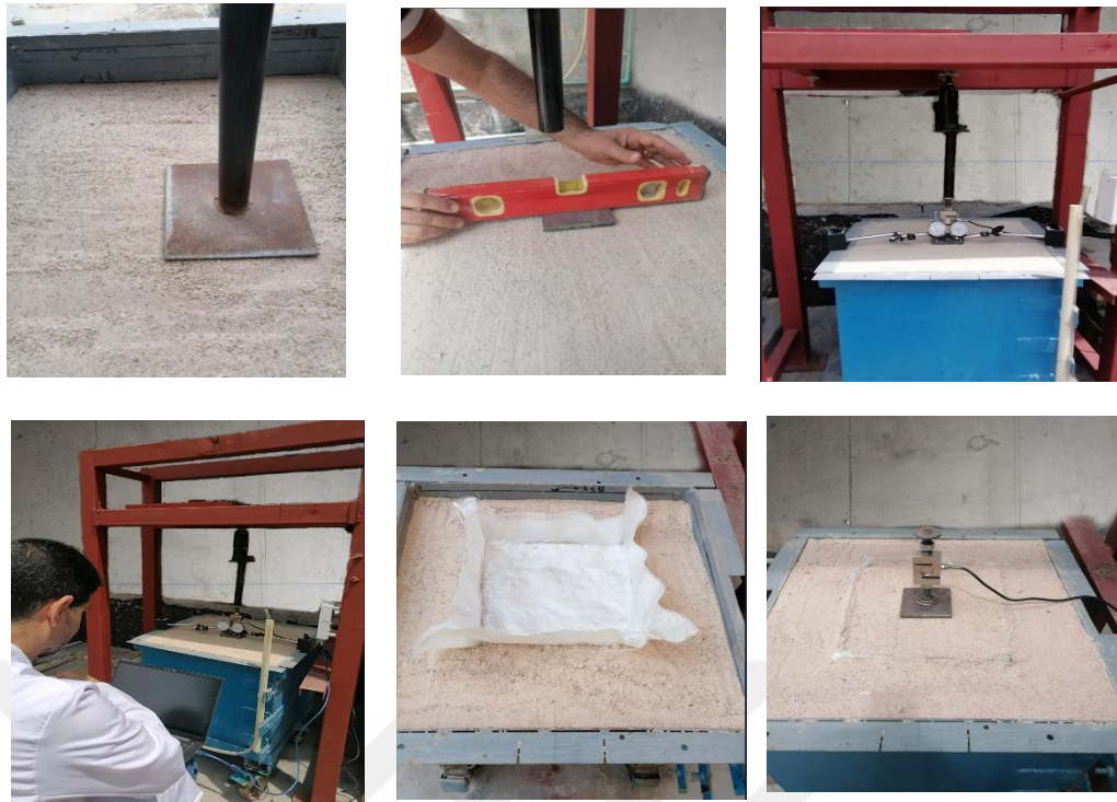
Plate 3.8 Preparing to place the soil and test at a dry state
