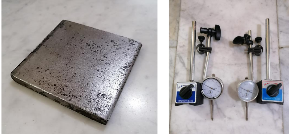
Plate 3.6 Square steel plate and dial gage
