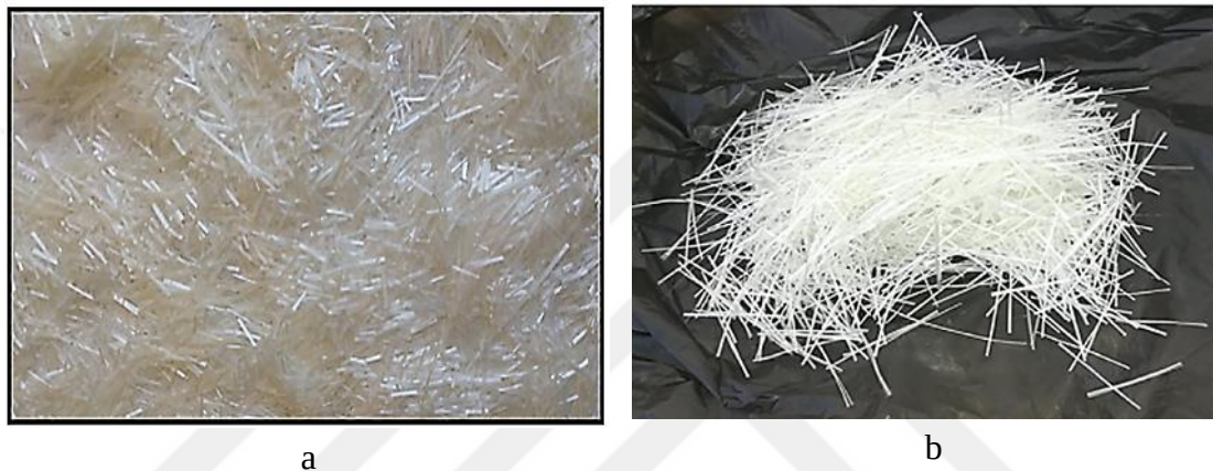
Figure 1.3 E-Glass fiber material a. Glass fiber used by A. Ateş, 2016 [33]. b. Glass fiber used by S. Rabab’ah, 2021 [34].
