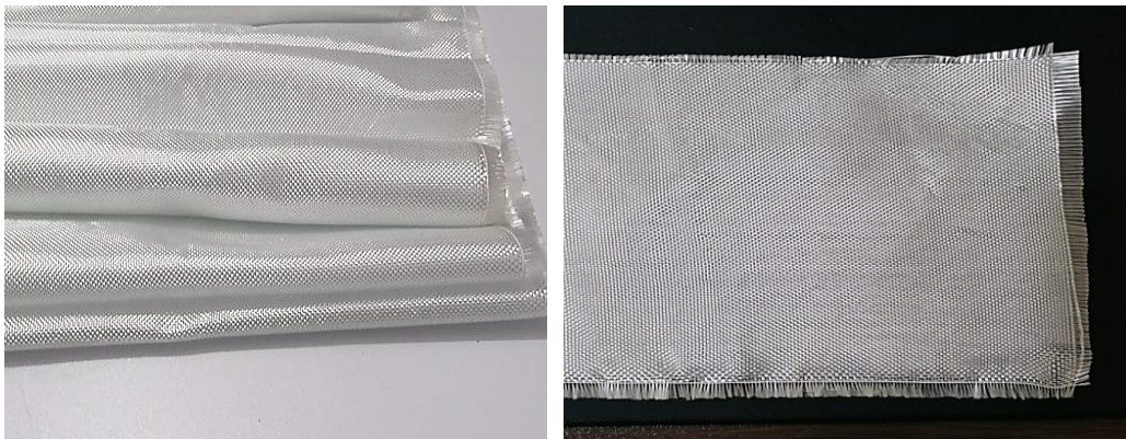
Plate 3.2 E-glass fiber fabric material used in this study
