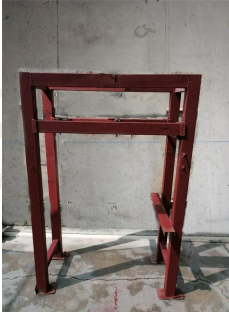
Plate 3.3 Steel load frame with axial load system.
