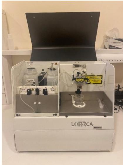
Şekil 15. Laser-assisted Optical Rotational Cell Analyzer” (LORCA, Mechatronics, Amsterdam, Hollanda)
