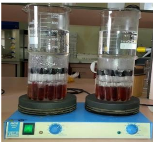
Figure 3.7. The boiling of sample tubes for tannin analysis
