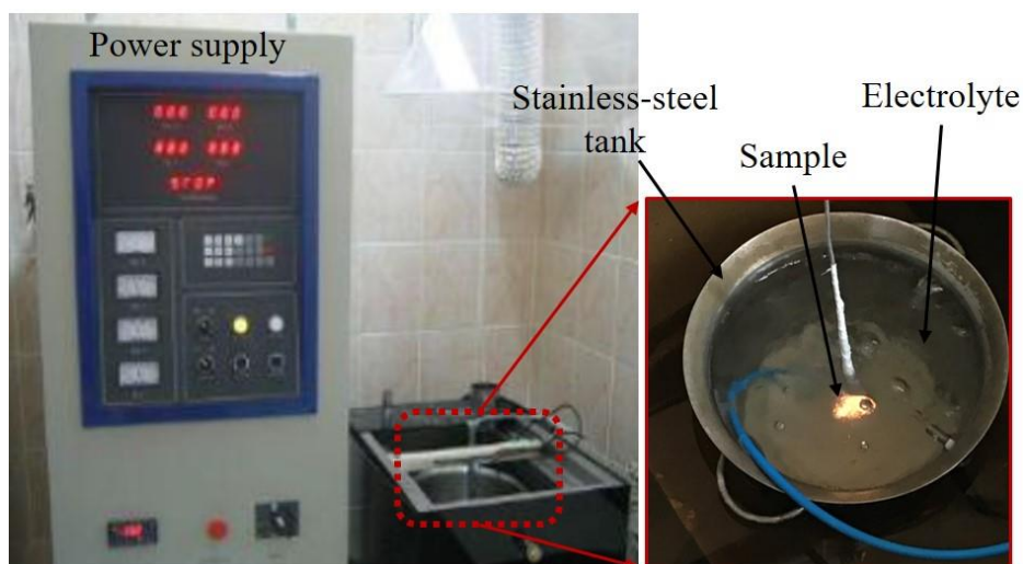
Figure 4.7: MAO unit and an example for spark formation on the sample during the process.
