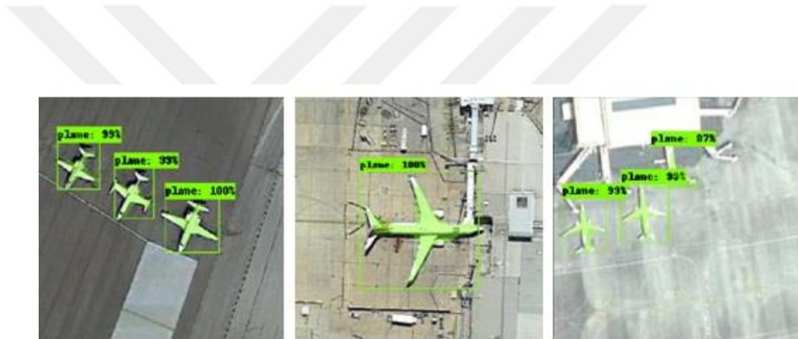
Figure 5.20: Detection samples - satellite images.
