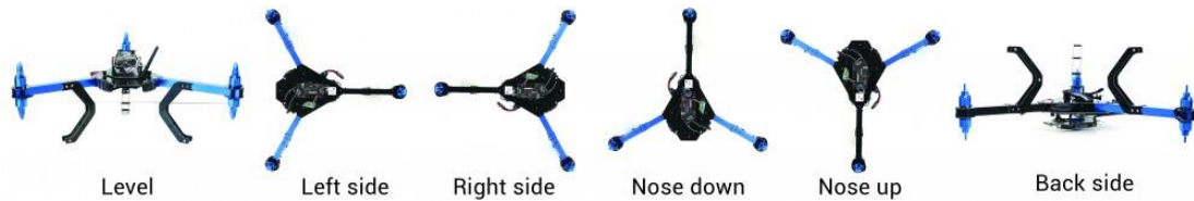
Figure 5.13 Full 360 degrees align process [46]
