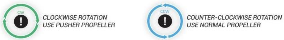
Figure 4.18 CW and CCW propeller rotation [46]
