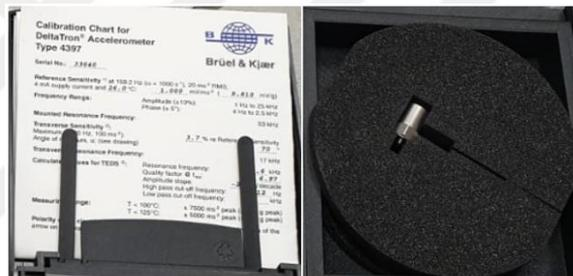
**Figure 3.5 :** Accelerometer B&K Type 4397 used in the experiments.
