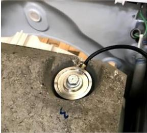
**Figure 3.19 :** Mounted load cell.
