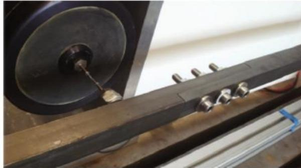
**Figure 1.8 :** Brake–Reuß beam excited by shaker [3].
