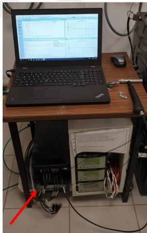
**Figure 2.11 :** Multichannel FFT analyzer (bottom left) used in a hammer impact test.
