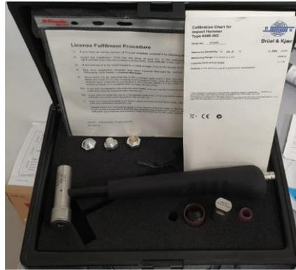
**Figure 3.4 :** Impact hammer B&K Type 8206 used in the experiments.
