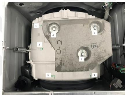
**Figure 1.16 :** Example of top counter weight assembly.
