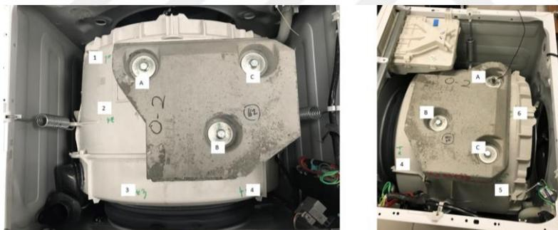
**Figure 3.3 :** Excitation points are denoted by numbers and measurement points are denoted by letters.
