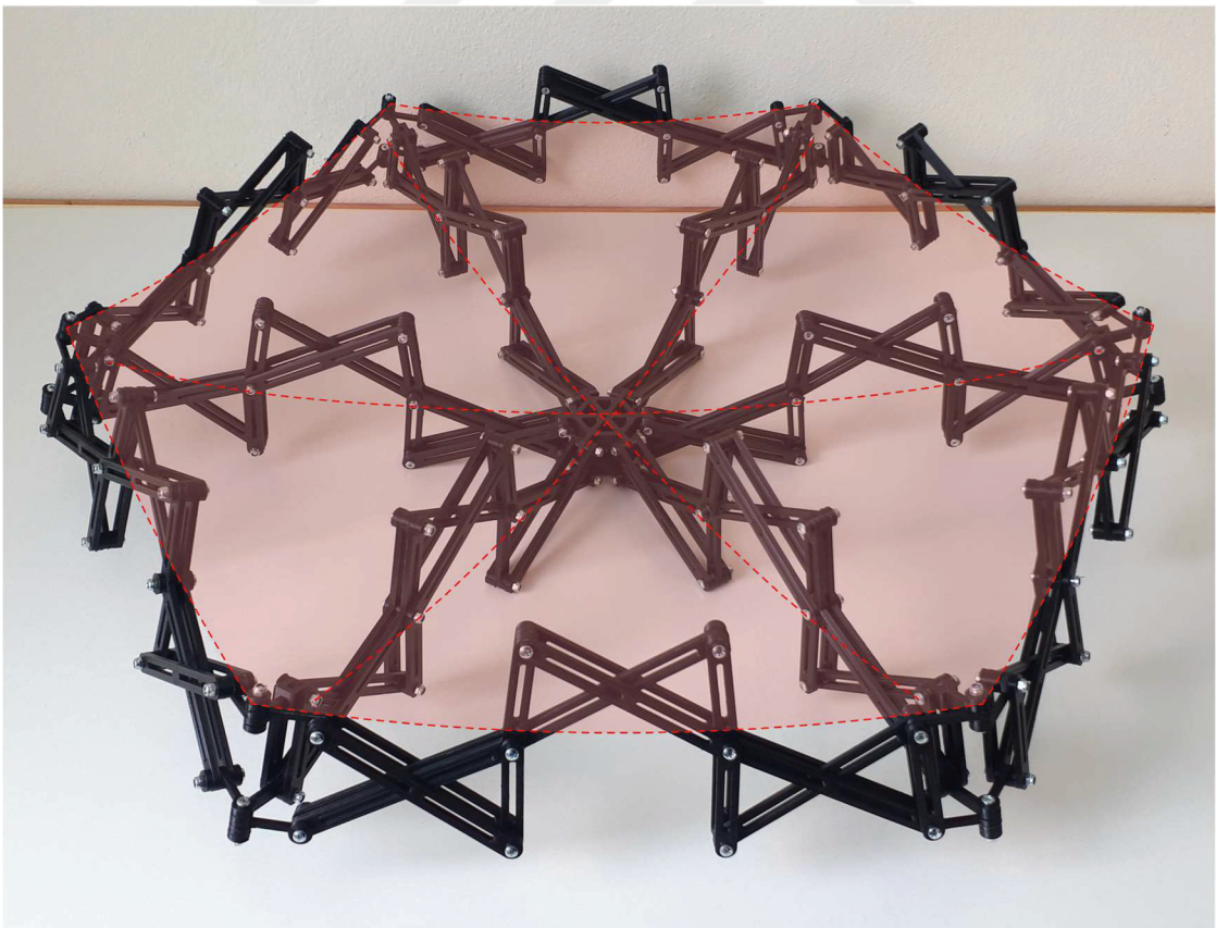
Figure 6.22. 3D Printed model of the transformable linkage when it is convex position.
