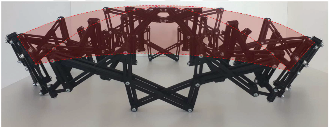
Figure 6.21. 3D-Printed model of the transformable linkage in a concave position
