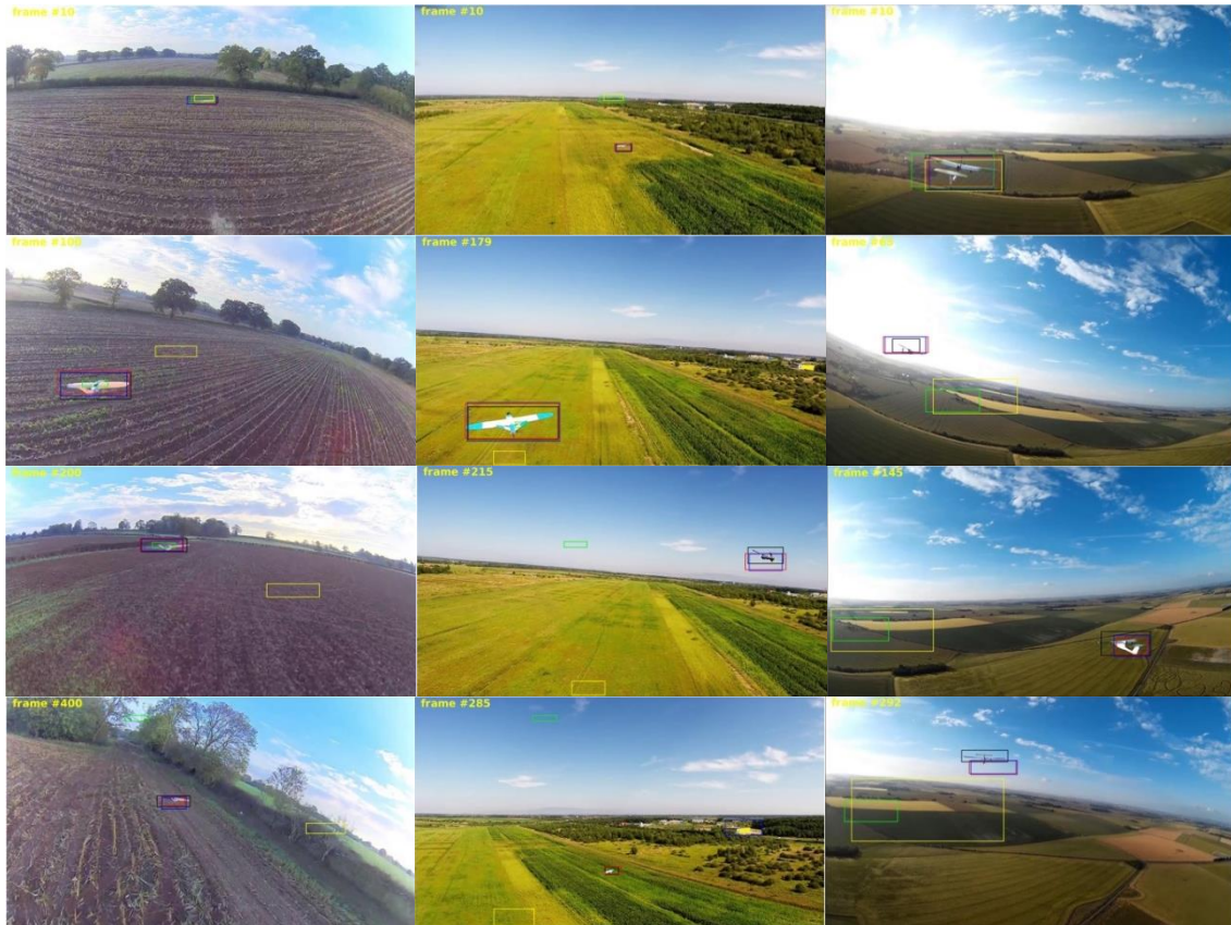
Image 4.2. A comparison of the proposed methods, UAVH (red bounding boxes), UAVH-Tiny (blue bounding boxes) with other trackers including CSRT (green bounding boxes), KCF (yellow bounding boxes) on the UAV Tracking dataset (Black bounding boxes shows ground-truth)
