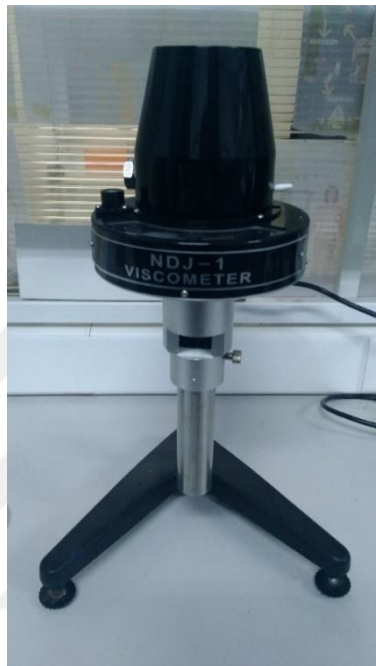
Figure 2.2. The experimental setup for viscosity measurement of precursor inks
