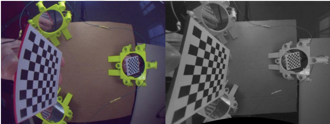
Figure 4. 7. A fisheye image on the left and an undistorted image on the right.
