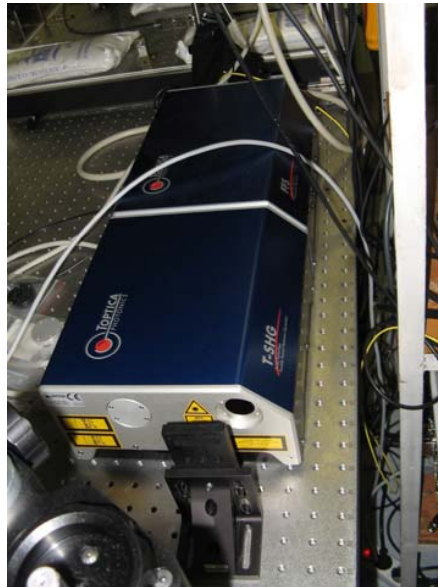
Fig.2.7. Er-doped fiber laser amplifier system
