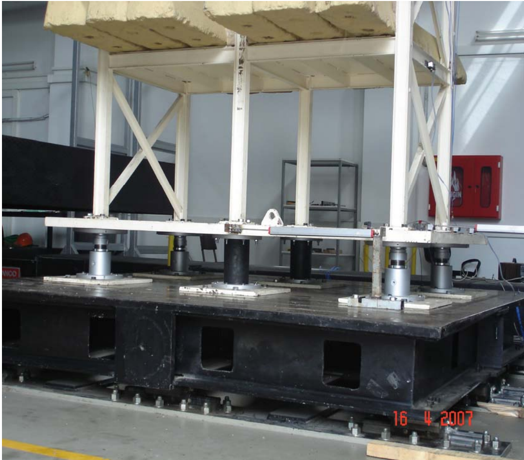
Figure 7.3. Configuration of isolators
