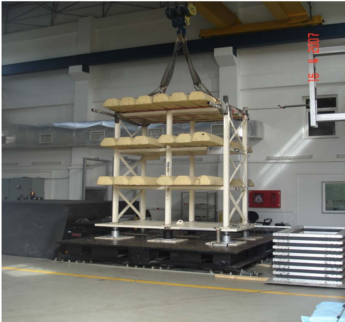
Figure 7.2. Passive Hybrid Isolation System
