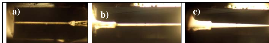
Figure 4.4: Images of the hall probe and its reflection from the sample surface: a) from the first side after get parallel to the surface, b) from the second side after get parallel to the surface, c) after the tilt angle is given.
