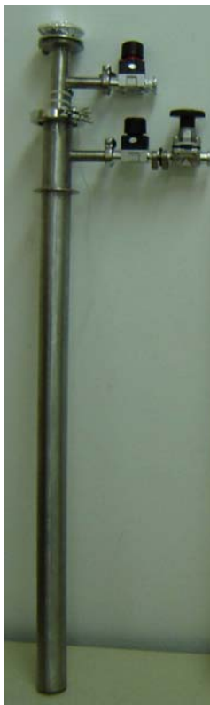
Figure 2.6: Our homemade cryostat system which is directly inserted to the liquid nitrogen tank.
