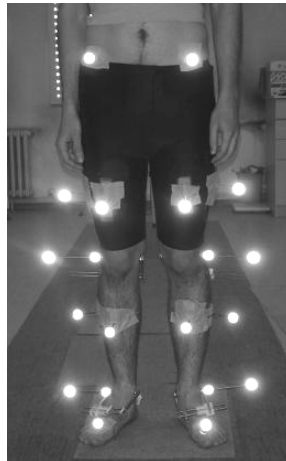
Figure 5.2 Static Shot with Front and Side Markers
