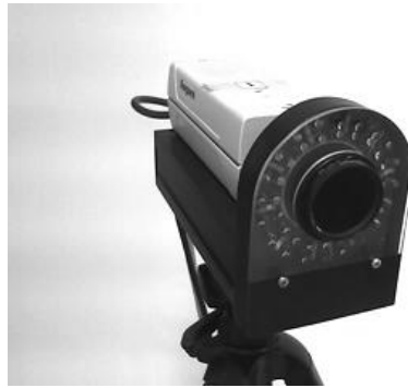
Figure 3.2 Camera with Infrared LED's and Filter
