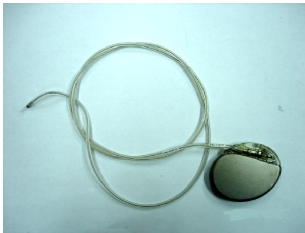
Figure 1. The photography of a typical active implantable medical device. The device shown in the figure is a pacemaker (Regency SC+ 2402L, Pacesetter, Switzerland).
