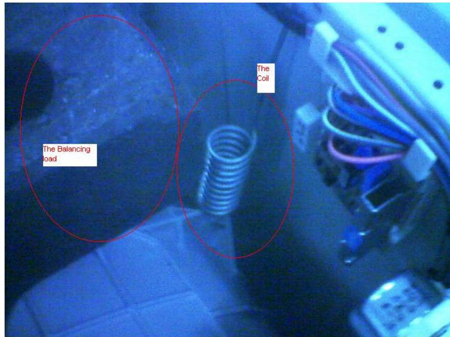
Figure 6.2- The coil and the balancing load of a washing machine
