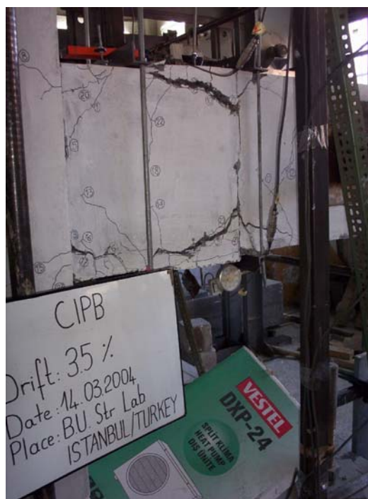
Figure 4.11. Crack distribution of specimen CIPB at 3.50 per cent story drift
