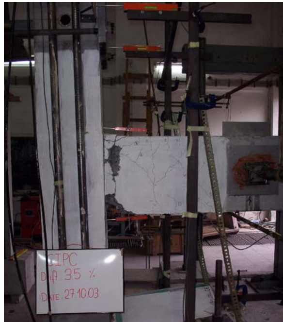
Figure 4.7. Crack distribution of specimen CIPC at 3.50 per cent story drift
