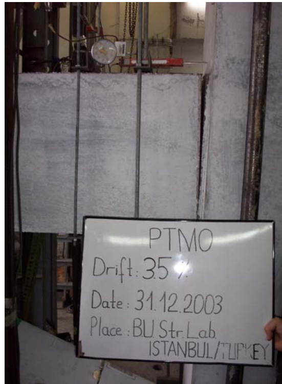
Figure 4.24. Damage level of specimen PTM0 at 3.50 per cent story drift
