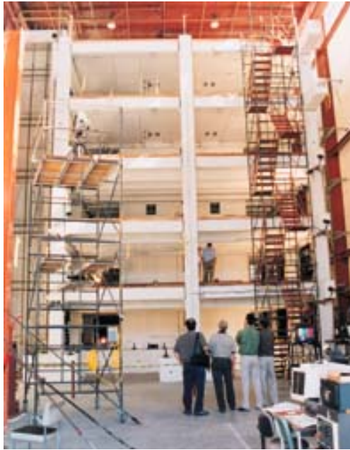
Figure 2.9. Prototype five story precast structure [38]
