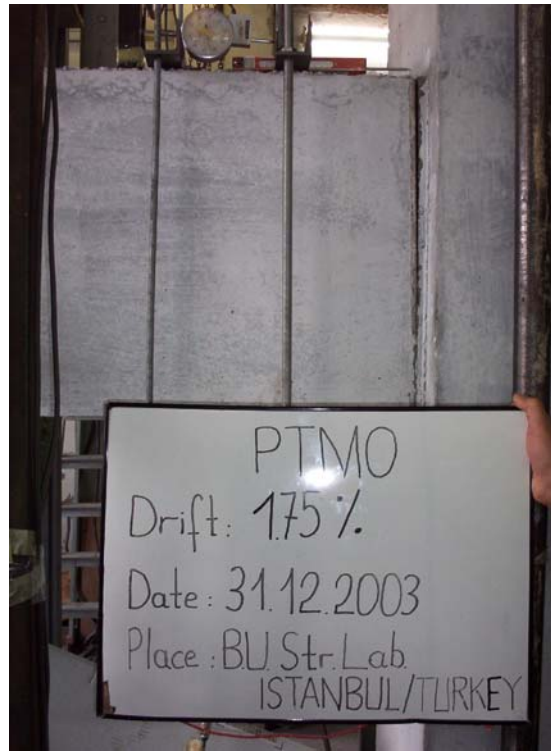
Figure 4.23. Damage level of specimen PTM0 at 1.75 per cent story drift
