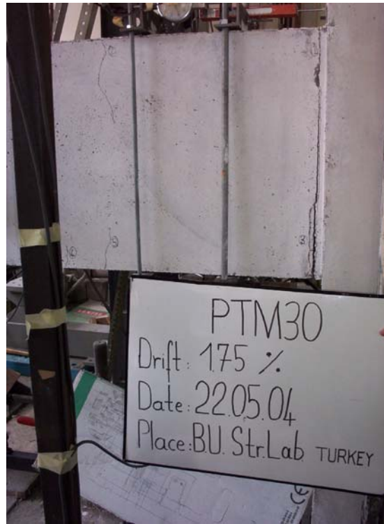
Figure 4.31. Damage level of specimen PTM30 at 1.75 per cent story drift
