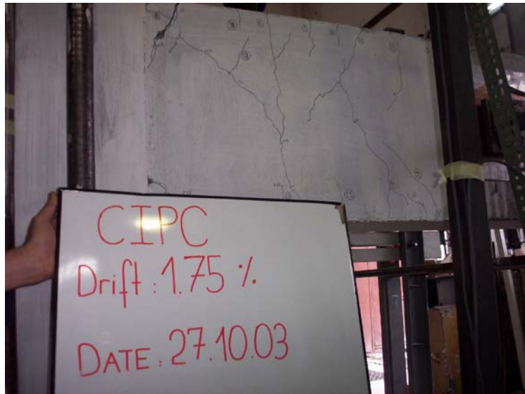
Figure 4.6. Crack distribution of specimen CIPC at 1.75 per cent story drift
