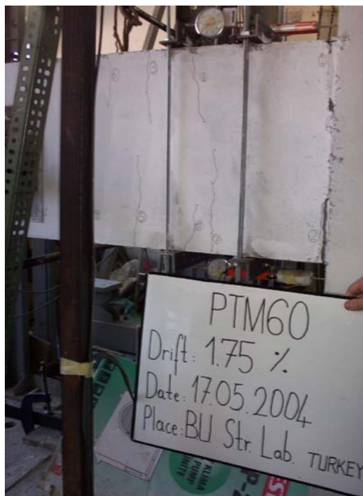
Figure 4.39. Damage level of specimen PTM65 at 1.75 per cent story drift
