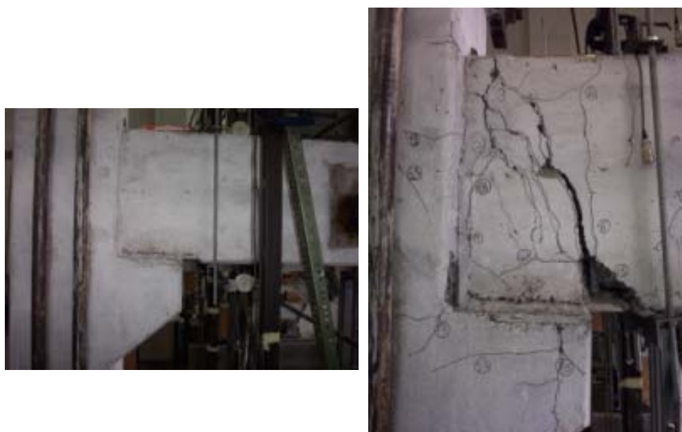
Figure 5.6. Damage level of specimen GOK-W
