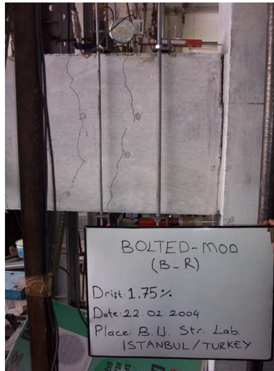
Figure 4.19. Crack distribution of specimen Mod-B at 1.75 per cent story drift
