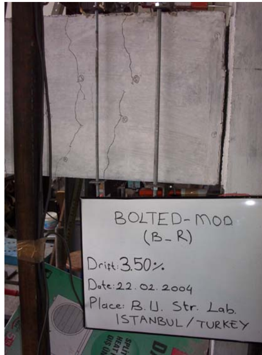
Figure 4.20. Crack distribution of specimen Mod-B at 3.50 per cent story drift
