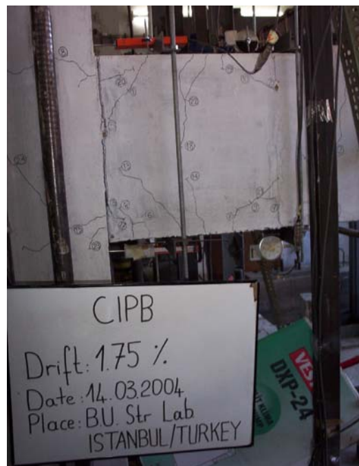
Figure 4.10. Crack distribution of specimen CIPB at 1.75 per cent story drift
