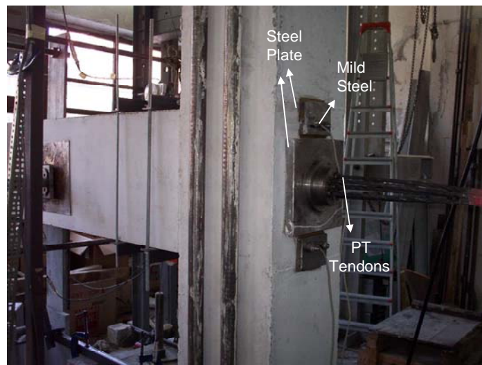
Figure 3.16. Assembled post-tensioned connection
