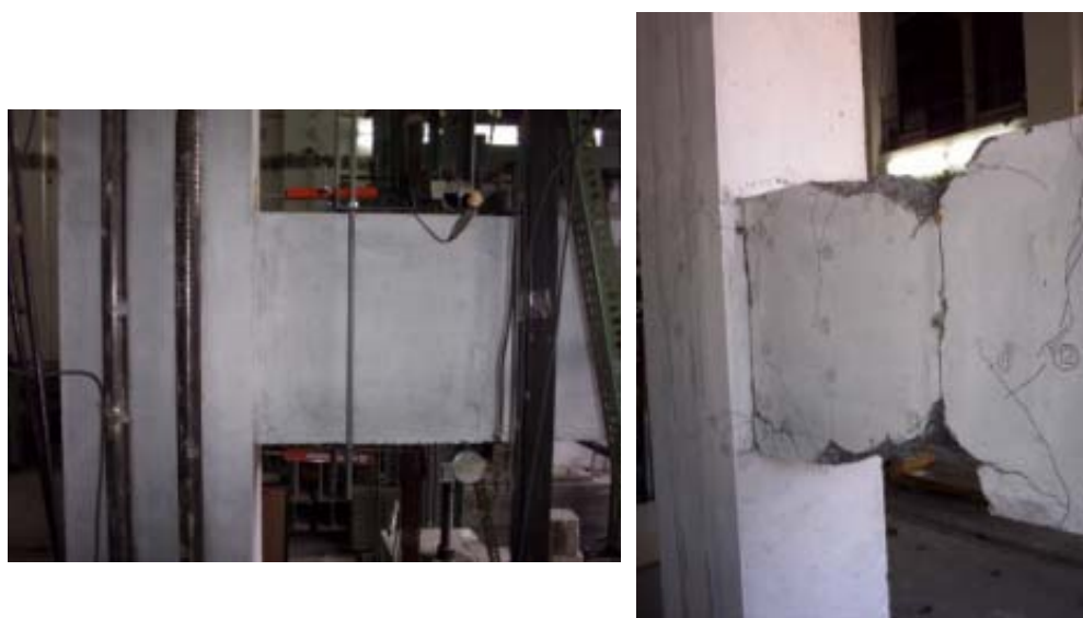
Figure 5.5. Damage level of specimen CIPB
