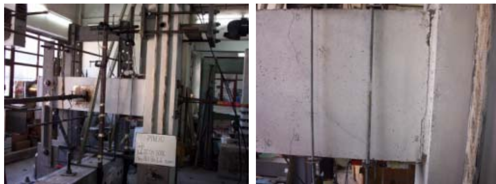
Figure 5.10. Damage level of specimen PTM30
