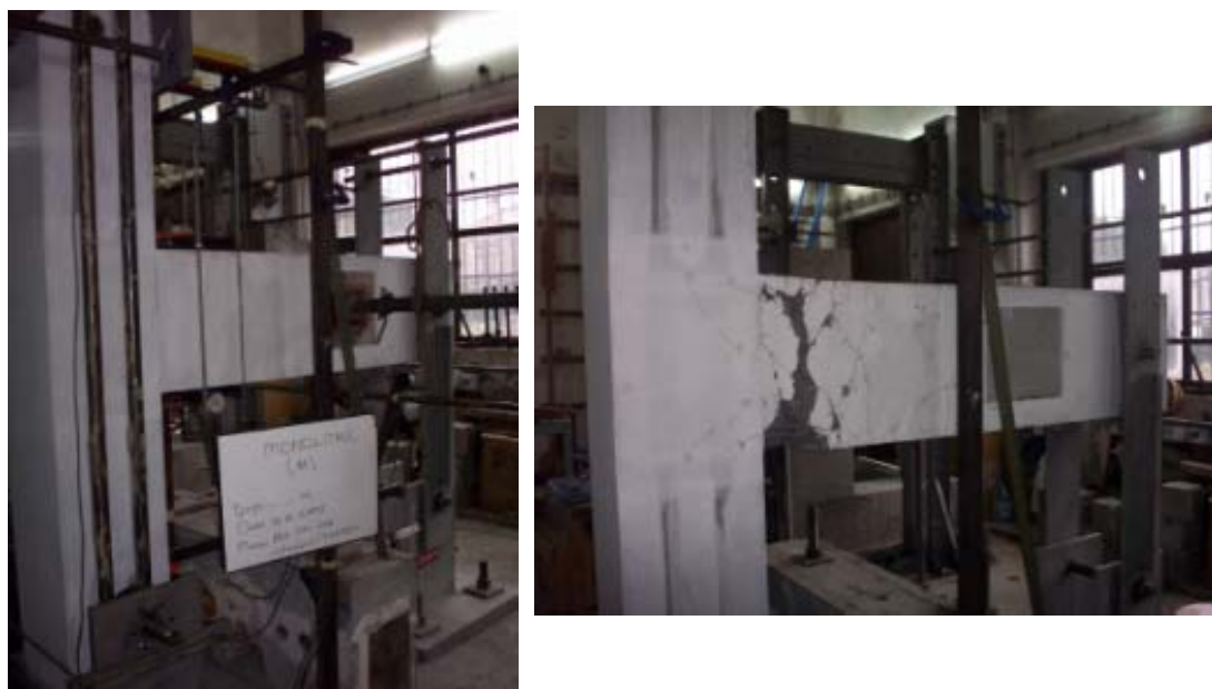
Figure 5.3. Damage level of specimen M
