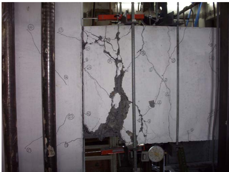
Figure 4.2. Crack distribution of specimen M at 3.50 per cent story drift
