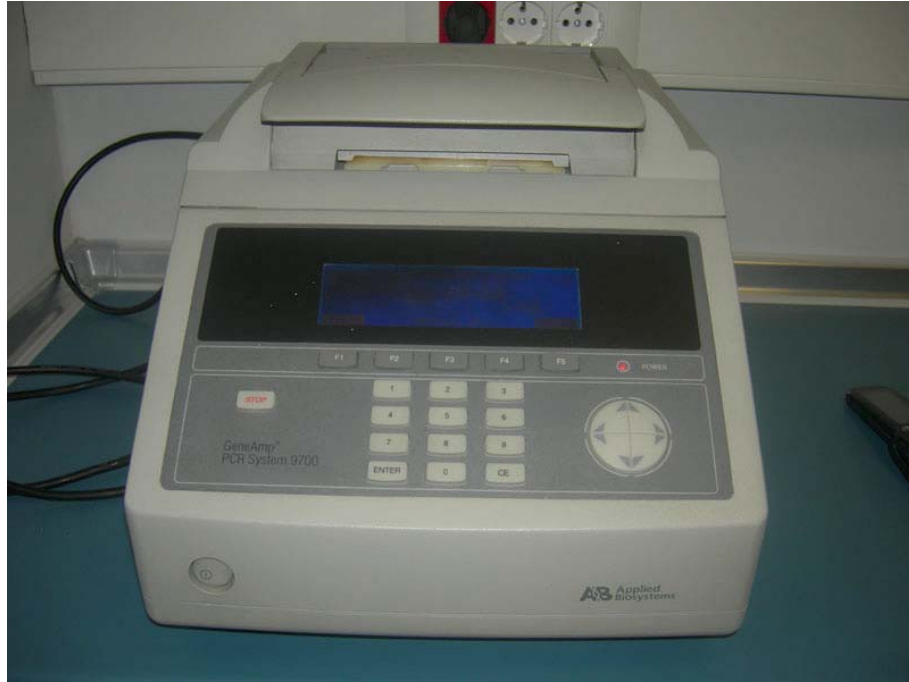
Resim 8. Thermal Cycler, PCR Cihazı (Applied Biosystems, GeneAmp, PCR System 9700)
