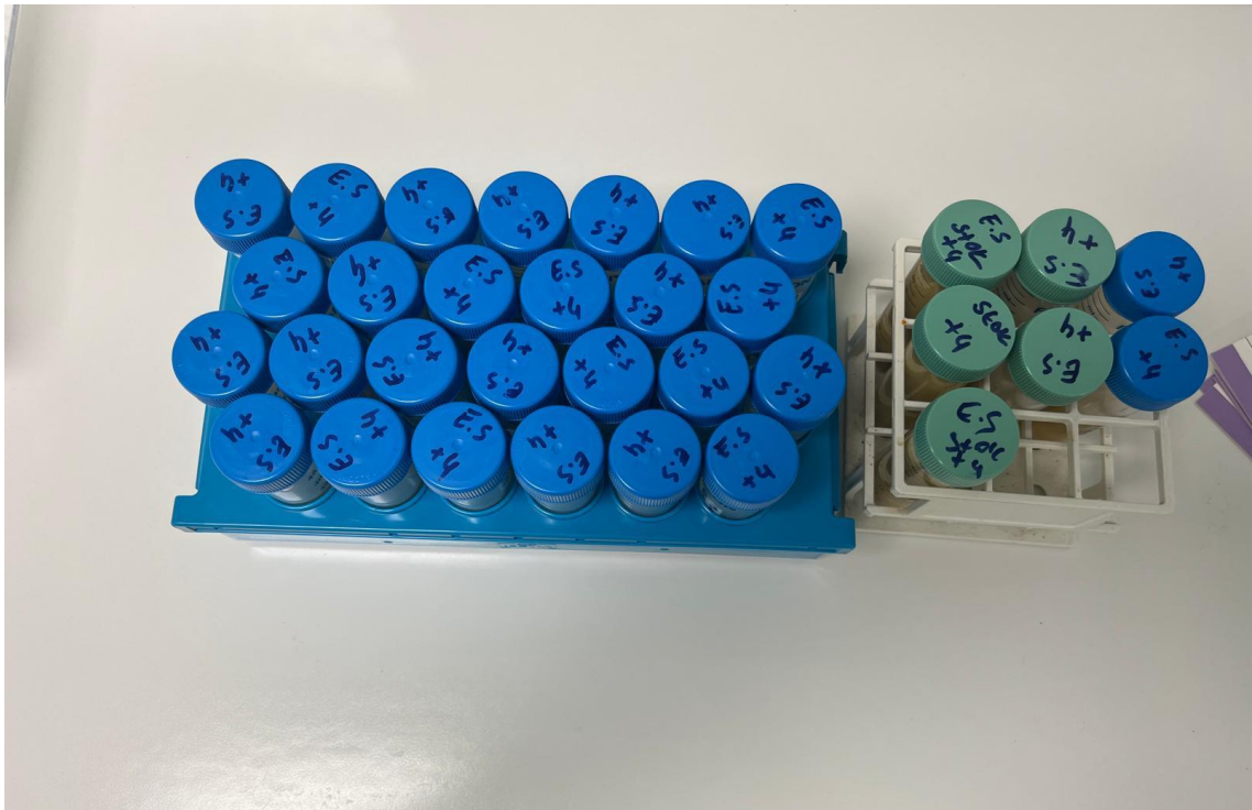
Figure 3.5. Falcon tubes prepared to be vortexed one per day and containing hesperidin and its solution ready to be placed in the refrigerator
