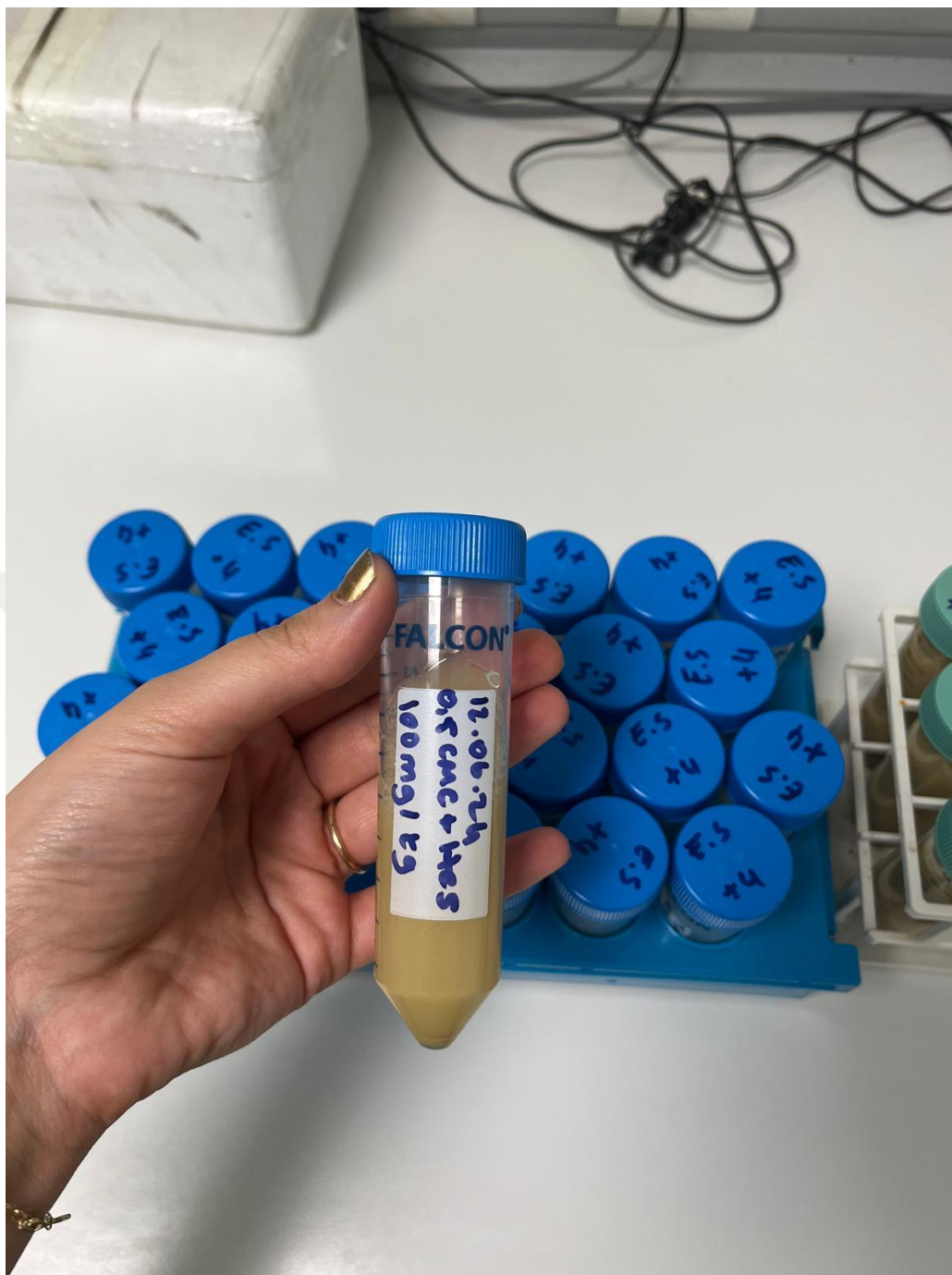
Figure 3.4. After mixing Hesperidin with CMC (carboxymethyl cellulose) and placing it in falcon tubes, labeling and sequential preparation for 28 days
