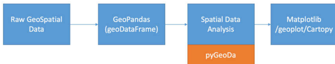
Figure 6.1. The Workflow Diagram of Geospatial Data in Python
