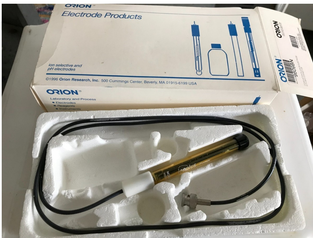
Figure 3.10. Fluoride measurement electrode (Thermo Scientific Orion 9609BNWP)
