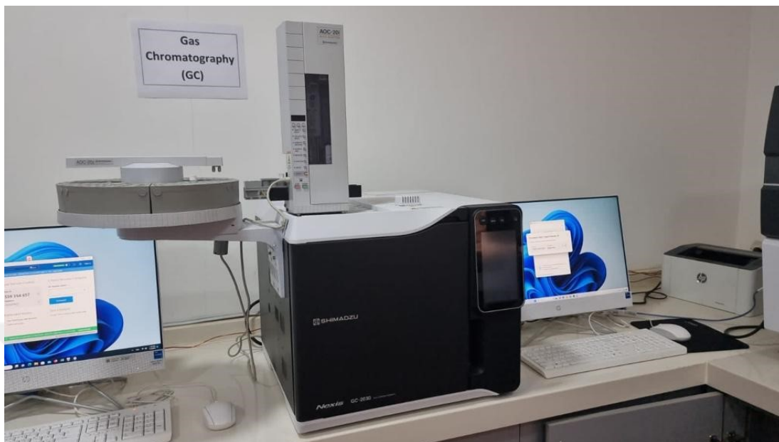
Figure 3.3. Gas Chromatography With Flame Ionization Detection (GC-FID) For Total Petroleum Hydrocarbon Analysis
