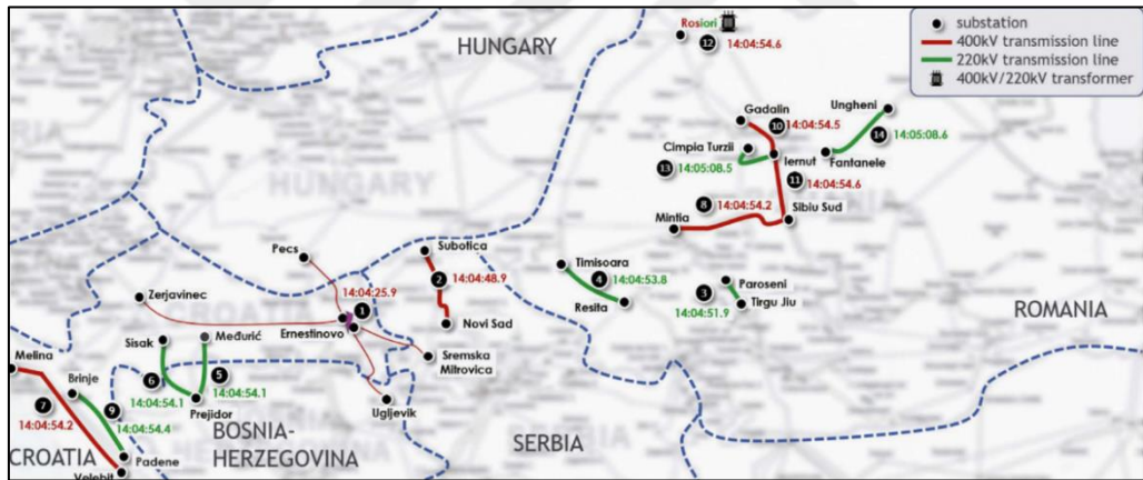
Figure 2.3. The sequence of events causing the system split in January 2021
